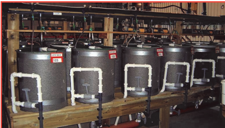
Figure 1. Experimental start feeding units with water and air temperature control. Photo: Nofima Marin AS
